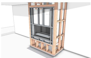
In this scenario an additional lightweight steel frame is used on the front face to support the wall linings and finishes.
