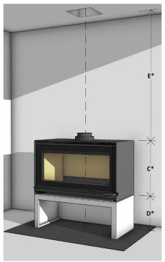
Install the fireplace on a plinth, base or preformed heat resistant structure following the TFS1000 Installation Manual. Fix the fire to the plinth, base or structure and the plinth or base to the floor. It is recommended that only HHA approved/accredited tradespeople should be used to install this fireplace. **\*See appliance dimensions over page.**
