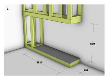
Build the chimney framework with consideration to flue pathways and meet the minimum fireplace opening requirements (850mm H x 1320mm W x 365mm D). Ensure a continuous base for the fireplace.
