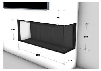
Attach wall linings to the framework and fireplace, maintaining a 3mm gap from the fireplace trim. Follow the provided wall lining cutout dimensions above for 13mm wall linings. Complete the project by adding additional finishes or fixtures.
