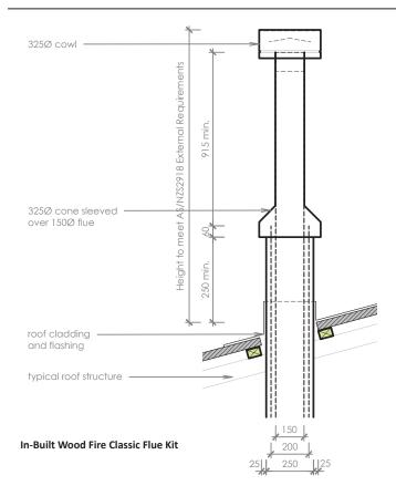
Install in accordance with AS/NZS2918 and the Escea TC950 Install Manual.
