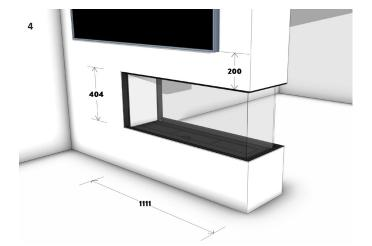
Attach wall linings to the framework and fireplace, maintaining a 3mm gap from the fireplace trim. Follow the provided wall lining cutout dimensions above for 13mm wall linings. Complete the project by adding additional finishes or fixtures.
