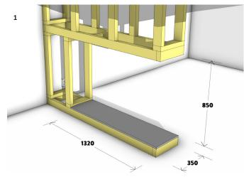
Build the chimney framework with consideration to flue pathways and meet the minimum fireplace opening requirements (850mm H x 1320mm W x 350mm D). Ensure a continuous base for the fireplace.
