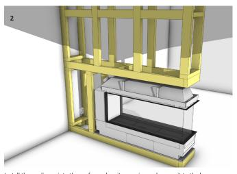
Install the appliance into the preformed cavity opening and secure it to the base. Ensure the fireplace is flush with the framework.
