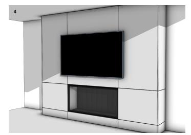
Fix the wall linings to the framework and the fireplace leaving a 1/4" gap to the glass opening. The wall lining can be bonded directly to the fireplace. vvlnstall any additional finishes or fixtures to complete the project.
