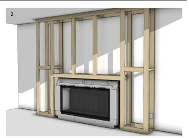
Install the appliance into the preformed opening in the chase. Secure to the framework using the supplied nailing flanges. The fireplace should be flush with the wood framing.
