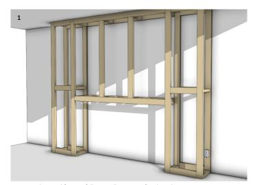
Construct the wood framing following all minimum fireplace chase opening requirements and with consideration to vent pathways. Provide a continuous base for the fireplace. Allow for mains power connection and an accessible isolation switch.
