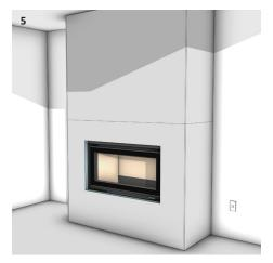
Fix the non-combustible fibre cement sheet substrate to the framework. All substrates, wall linings and finishes to the front face of the cavity must be non-combustible.
