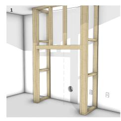
Select fireplace location and obtain flue centreline to ensure the flue run is clear from obstructions. Provide an electrical supply adjacent, with an isolation switch outside the cavity. Build the framework to the required dimensions and provide the Zero Clearance Kit vent inlet to the exterior.
