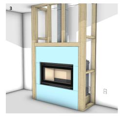
Install the flue and liners to the correct configuration and height. Cut, prime, and fix the Skamotec panels in place.
