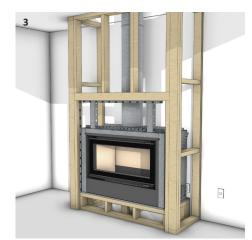
Install the fireplace onto a base or structure following the TC950 Installation Manual. Restrain the fire to its base. Fit the top panel and standoffs for the Zero Clearance Kit. Install the Skamotec fixing brackets to the perimeter of the cavity opening.
