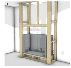
Install the structural base for the fireplace **40mm** behind the face of the timber framing. Build the sides, base and rear of the Zero Clearance Kit and install into the cavity.
