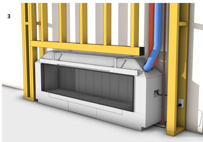
Install the appliance into the preformed cavity opening and secure it to the base. Ensure the fireplace is flush with the framework. Install electrical, network connections, and gas supply. Connect flue pipes to the fireplace and create the flue pathway to the terminal. Connect Powerflue electrical cable at both ends.
