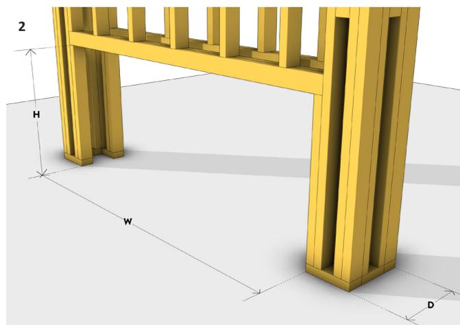
For a double sided installation build the chimney framework as above (2087mm W x 850mm H x 350mm D). Ensure a continuous base for the fireplace.
