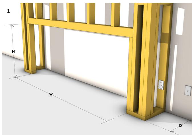
Build the chimney framework with consideration to flue pathways and meet the minimum fireplace opening requirements for a single sided installation (2087mm W x 850mm H x 365mm D). Ensure a continuous base for the fireplace.
