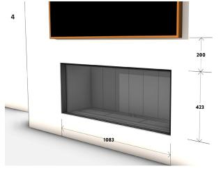
Attach wall linings to the framework and fireplace, maintaining a 5mm gap from the fireplace trim. Follow the provided wall lining cutout dimensions above for 10mm wall linings. Complete the project by adding additional finishes or fixtures.
