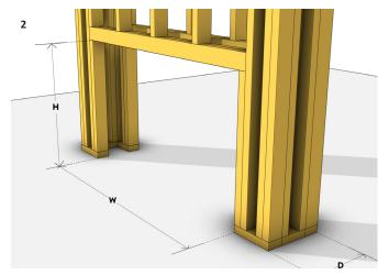
For a double sided installation build the chimney framework as above (1500mm W x 850mm H x 350mm D). Ensure a continuous base for the fireplace.
