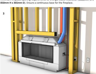
Install the appliance into the preformed cavity opening and secure it to the base. Ensure the fireplace is flush with the framework. Install electrical, network connections, and gas supply. Connect flue pipes to the fireplace and create the flue pathway to the terminal. Connect Powerflue electrical cable at both ends.
