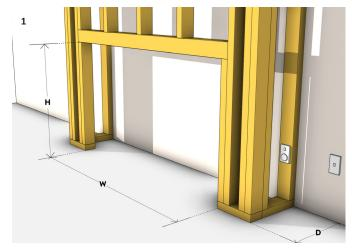
Build the chimney framework with consideration to flue pathways and meet the minimum fireplace opening requirements for a single sided installation (1500mm W x 850mm H x 365mm D). Ensure a continuous base for the fireplace.
