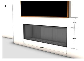
Attach wall linings to the framework and fireplace, maintaining a 5mm gap from the fireplace trim. Follow the provided wall lining cutout dimensions above for 10mm wall linings. Complete the project by adding additional finishes or fixtures.
